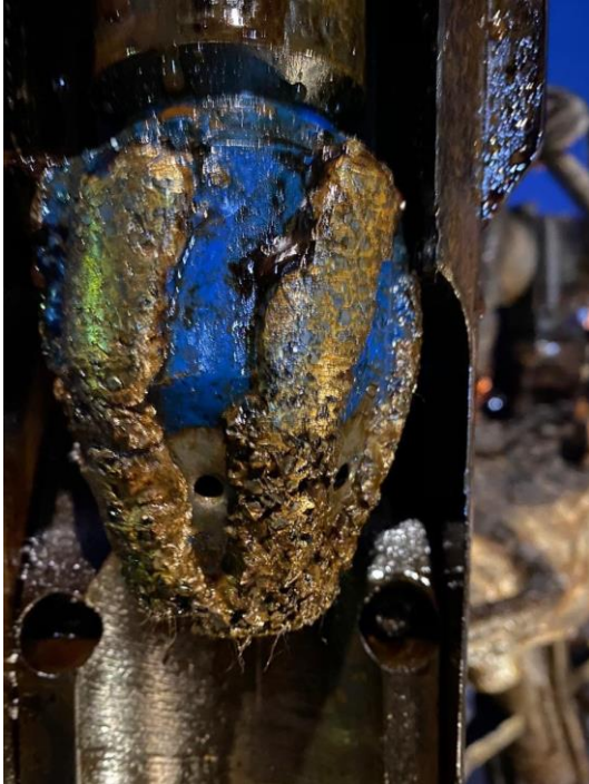
Figure 7 – Traces of oil on the mill
