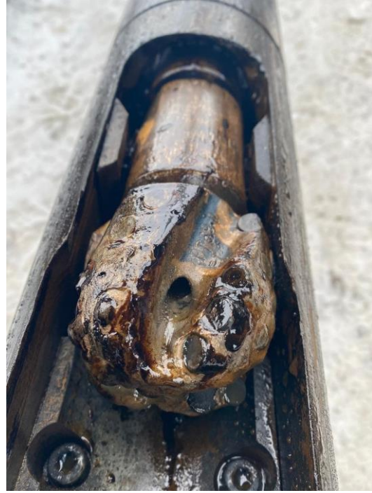
Figure 8 – Traces of oil on the drill bit
