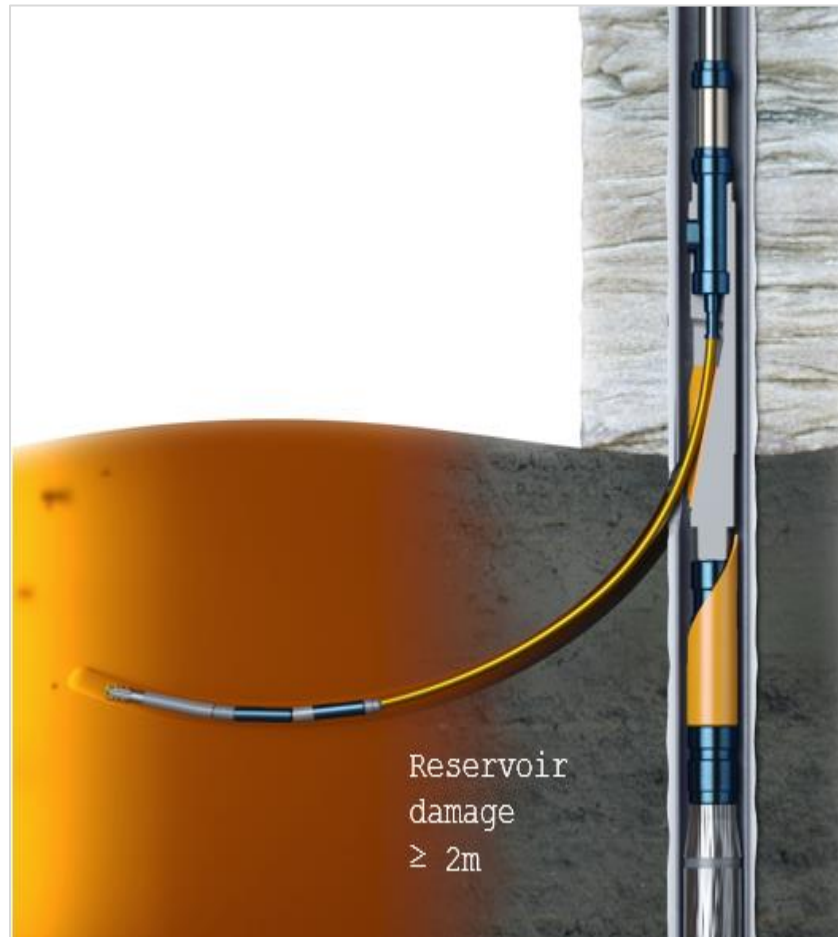
Figure 14 – Scheme of the radial drilling
