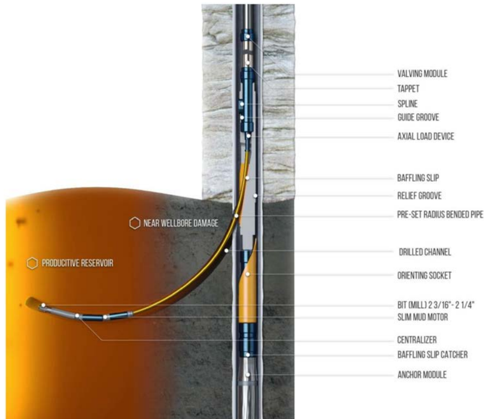
Figure 2—Main elements of TS
