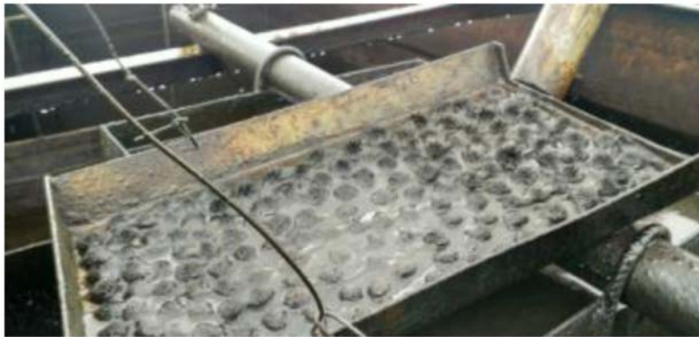
Figure 4—Cutting chips removal during the milling of the "window".
