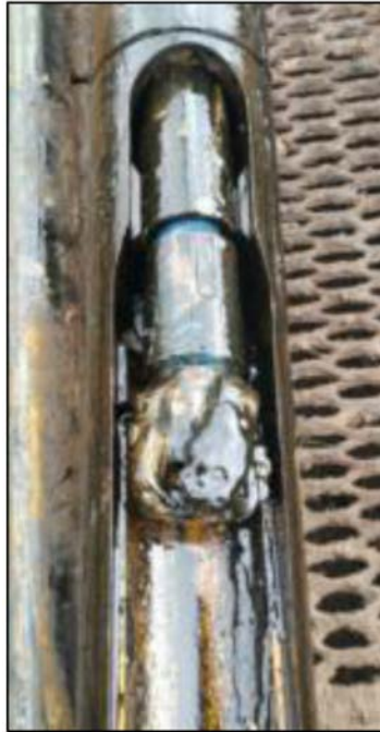
Figure 5—Condition of the drilling module after 14 m (46 ft) long channel drilling (traces of oil on the drilling module).
