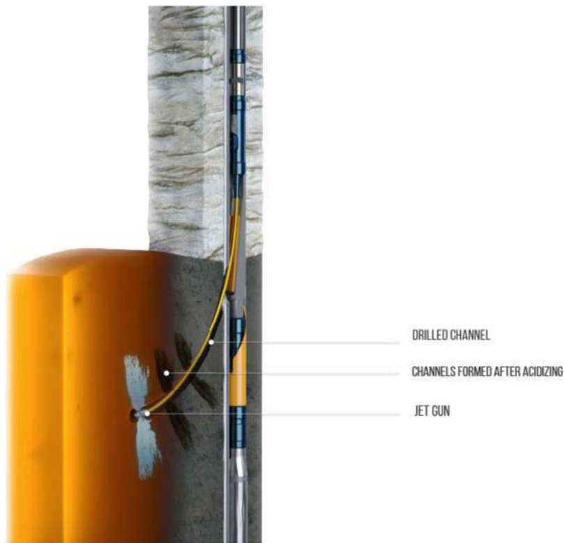
Figure 10—Acid treatment of the drilled channels
