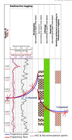
Fracture direction trend according to interpretation of electric microimager and cross-dipole sonic data
