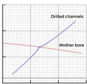
When compiling the design, the azimuth direction of the channels was oriented perpendicular to the regional stress
