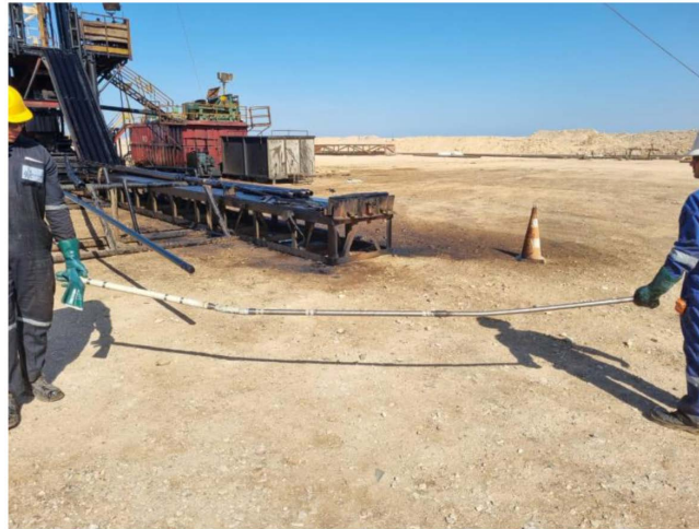
Figure 11—String of logging tools made-up at a rig site
