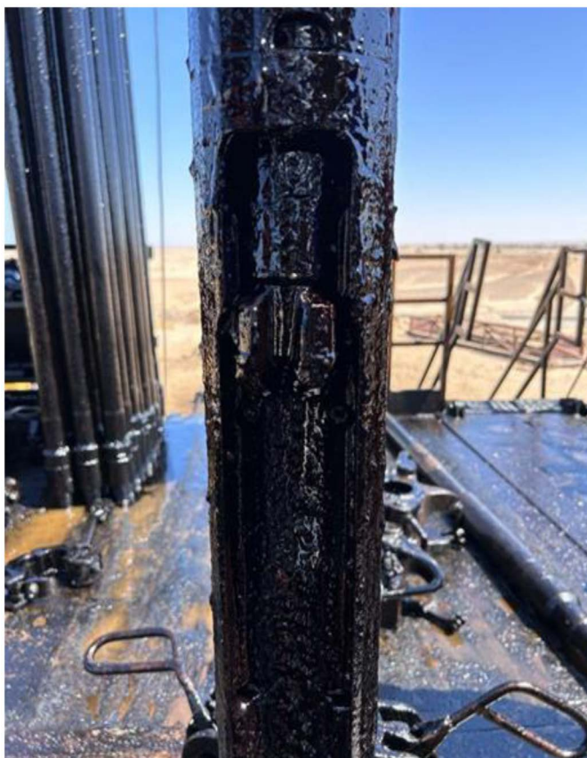
Figure 7—Mechanical Radial Drilling BHA after POOH
