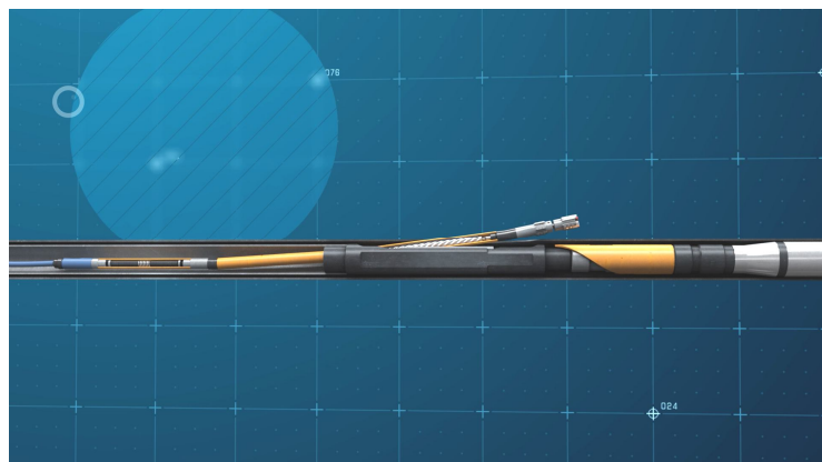
Fig. 2. TS «Perfobur» assembly in horizontal well
